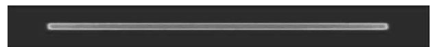
Figure 3: Energy distribution with fiber coupled line optic providing a laser focus of 160 x 4 mm
